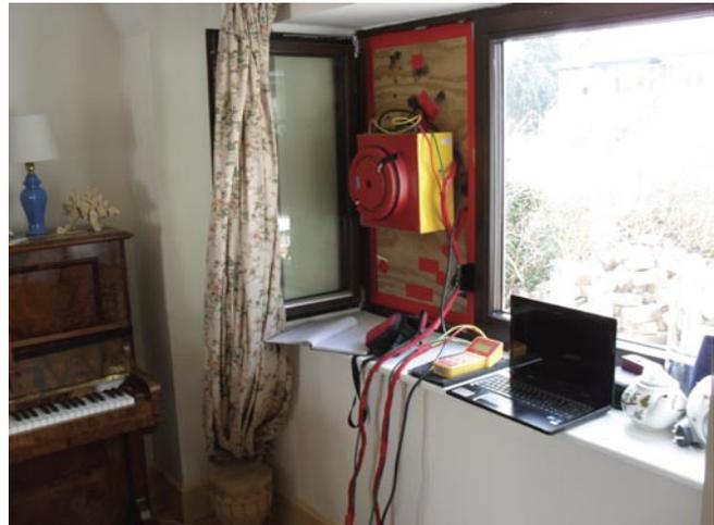
*Regardless of how well the work is carried out, every home has to be pressure tested after completion to ensure that no parts were omitted in error. The fan was mounted in a window so that all doors could be air tested properly.*
