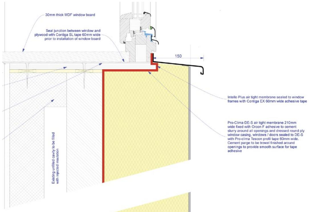
secondary airtight layer, important particularly for the floor-wall junction, but we realised that future-proofing required that, as far as possible, airtight elements should be difficult to reach and damage during future furniture installation and decorating works.
