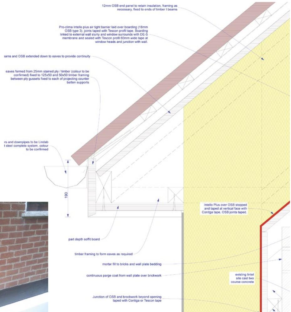
cannot sag under gravity or be damaged by people in the loft spaces. This crossover from the membrane inside (walls) to membrane outside (pitched roof) caused the logistical difficulties with membrane having to pass between the ridge beam and its support during the construction of the extension.
